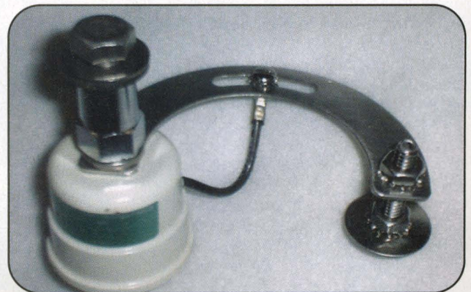
Photo C. A commercial 440-MHz vertically polarized DDRR antenna.
