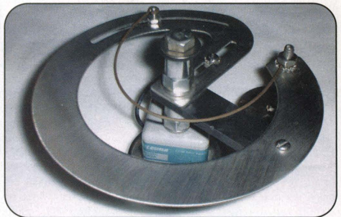
Photo B. A commercial 2-meter vertically polarized DDRR antenna.
