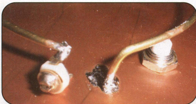
Photo I. Using a capacitor to lower the DDRR's frequency.
