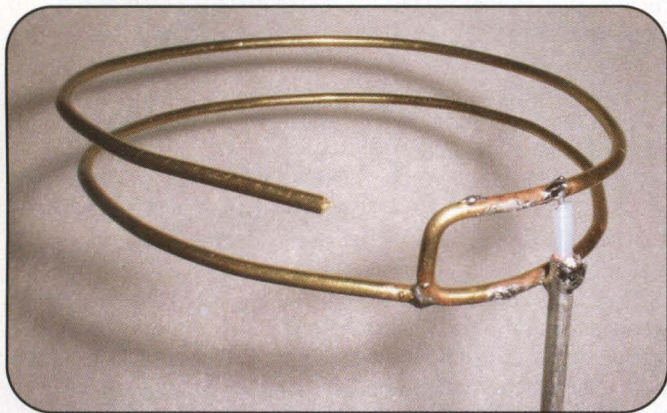
Photo H. Basic wire DDRR antenna.
